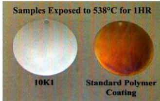
The diagram demonstrates the ability of Magnaplate 10K to withstand oxidation at elevated temperatures.
