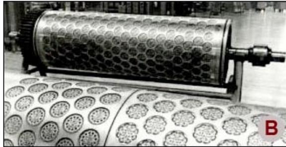
**B.** A cookie manufacturer eliminates frequent production downtime to change batter-clogged cookie molds and also reduces mold replacement by treating brass molds with an FDA/USDA/ AgriCanada-compliant NEDOX coating. Other food processors solve mold release, cleanup and sanitation problems by specifying NEDOX for molds, extrusion pistons and dies, filling nozzles, rollers, trays, kettles, and blades.
