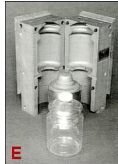
**E.** A NEDOX coating on the steel portions and the aluminium portions solved galvanic corrosion and erosion problems encountered on their combination steel/aluminium molds used to injection blow-mold PET bottles. The coatings also prevented corrosion created by condensation on both metals.
