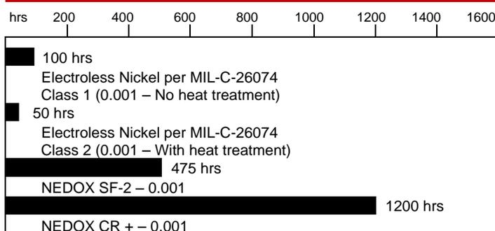
Hours of exposure in 5% NaCl until first appearance of corrosion spots per ASTM B-117
