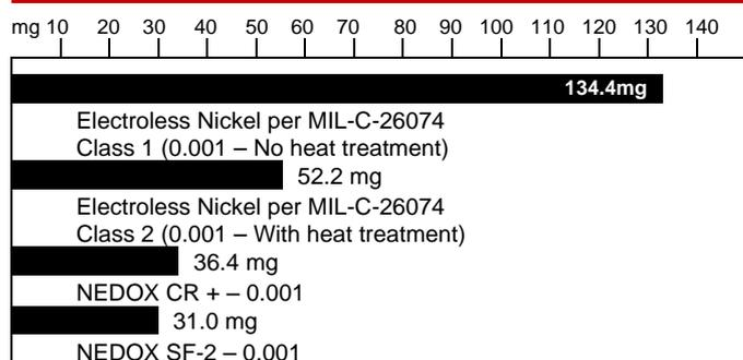
\* Weight loss = mg per 10,000 cycles – CS10 wheel using Taber Abrasion
