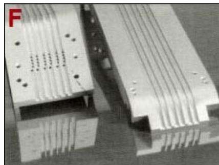
**F.** Guide plates used in pharmaceutical form/fill seal machine. NEDOX prevents product hang-up, keeping flow rates steady.
