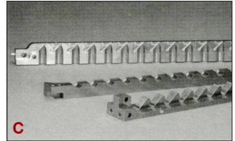
**C.** NEDOX was used on these lipstick mold parts to ease cleanup of residues left from the molding process. The smooth NEDOX surface increased product quality and appearance by minimizing pinholes and blemishes on the lipstick.
