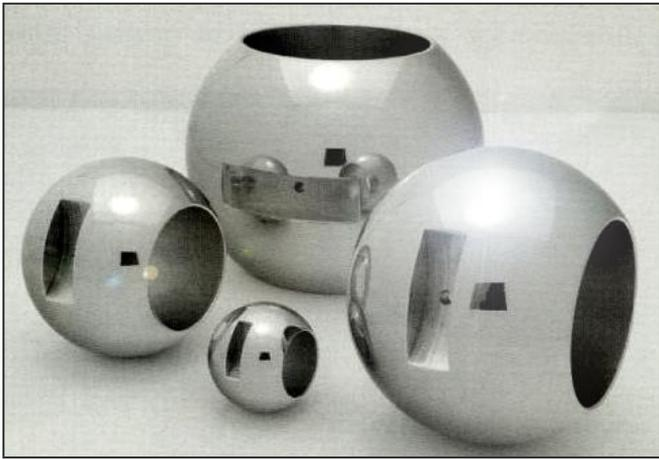
Because of its extremely low coefficient of friction, the HMF coating applied to the SS ball portion of a Worcester Controls valve containing a powdered metal seat, eliminates galling that could result in premature wear, leaking and, ultimately, total failure of the valve. In addition, use of the coating permits raising the operating temperature by over 200°F (93°C) and extends both the active life and shelf life of the valves by 50%.
